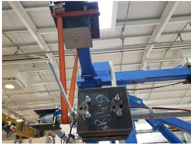
c. Fractured hanger rod at the end of the branch pipe.
