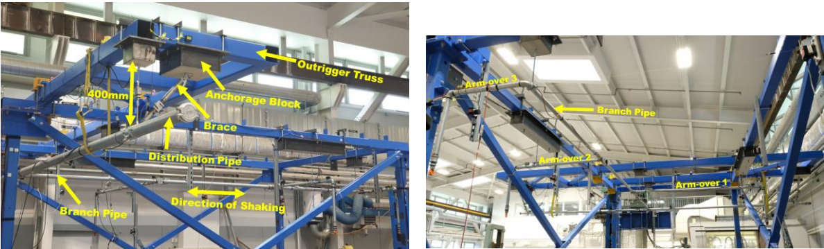
a. Actual image of the specimen mounted on the test frame.
