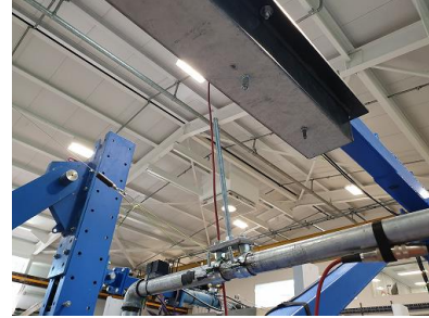
d. Fractured hanger rod at the end of arm-over 2.
