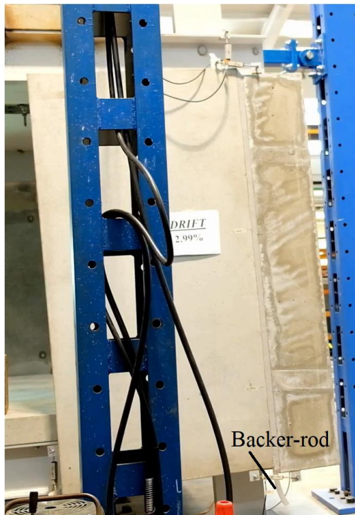
b. Return-cover corner sub-assembly
