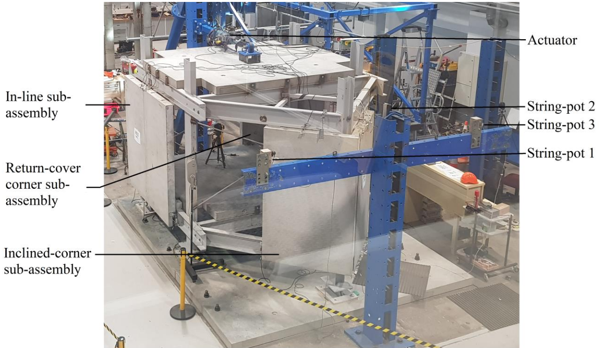
Fig. 2–Test setup, instrumentation, panel sub-assemblies
